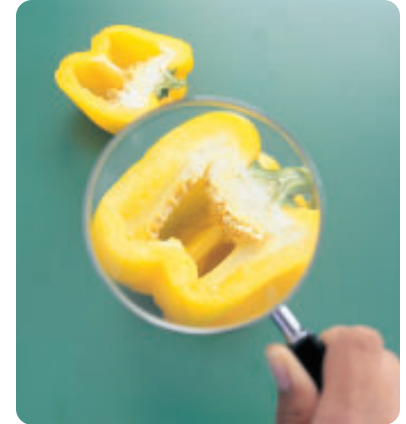
Figure 1 Lenses have a variety of uses, depending on their size, shape, and other properties. As light passes through this lens, it refracts to create enlarged images.
