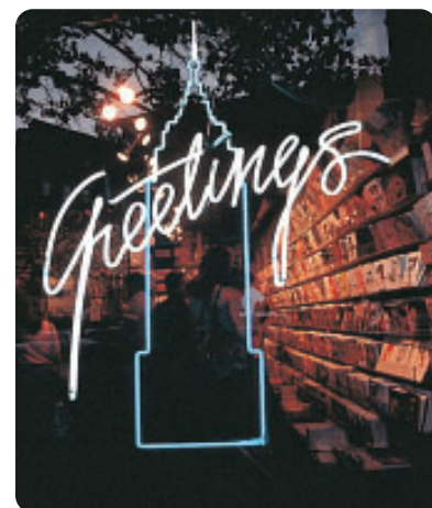
Figure 5 This artificial light source works because of electric discharge.
