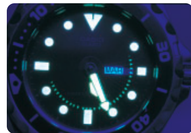
Figure 4 The painted luminous dials on some watches and clocks are phosphorescent.
