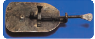
(a) Leeuwenhoek’s microscopes used a single lens mounted between two brass plates to magnify objects.
