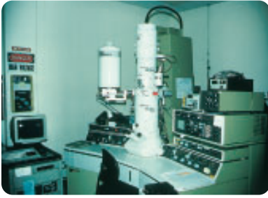
(a) The transmission electron microscope uses magnets to concentrate a beam of electrons and direct it at a specimen.
